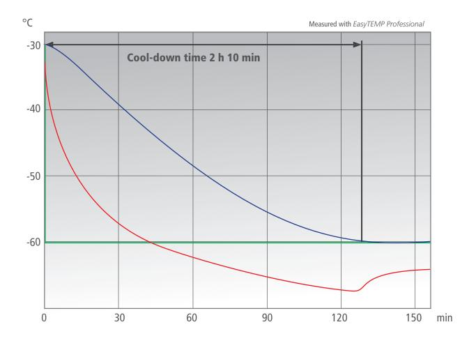
SetpointTemperature in reactor's interiorTemperature in reactor's jacket
